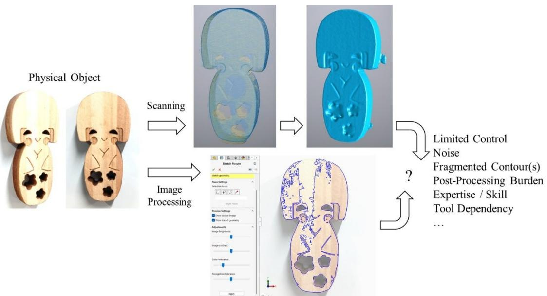
A non-contact structured-light 3D scanner (EinScan-SP, white-LED pattern projection; point spacing 0.17–0.20 mm) was used to digitize the object. As seen in the above figure, scanning the full object yields a dense point cloud of 186,873 points, resulting in a mesh of 498,670 triangles. However, the output exhibits significant distortions, including surface bumps, irregular hole-
